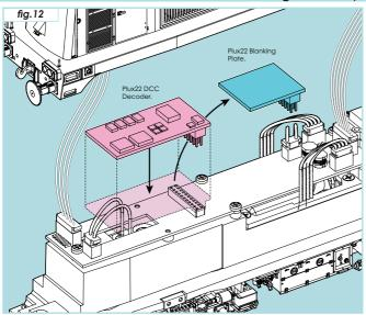
**4.** Remove the Plux22 Decoder Blanking Plate and Push fit your Plux22 Loco-Decoder (**36-570**) or DCC Sound Decoder (**Fig. 12**).
