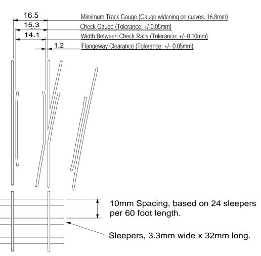
Rail Section Should Be a Minimum of Code 75
